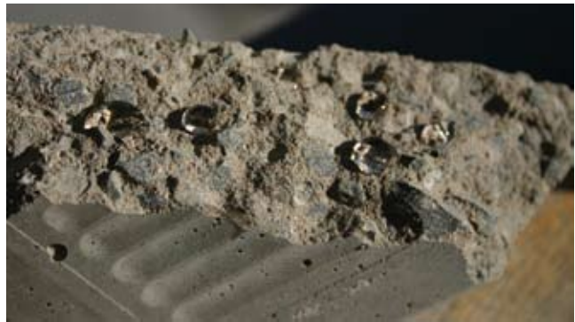
Photo 3. Concrete treated with a nanotechnology-based sealer repels water. Efficacy with friable mortars such as paving beds is not yet known.
