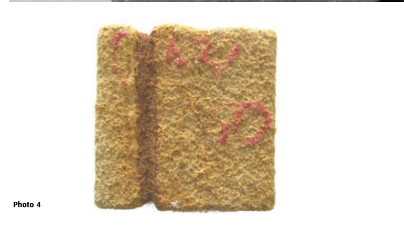
Photos 1 & 2: Comparison of natural contour delamination of sandstone and similar delamination on test specimens following salt attack test. Photo 3: The pattern of the adhesive applied to the rear of the panel, which allowed transmission of the salt solution, has been highlighted by the subsequent attack and decay. Photo 4: The salt attack can identify less durable components of stone as seen by the preferential decay of the darker band.
